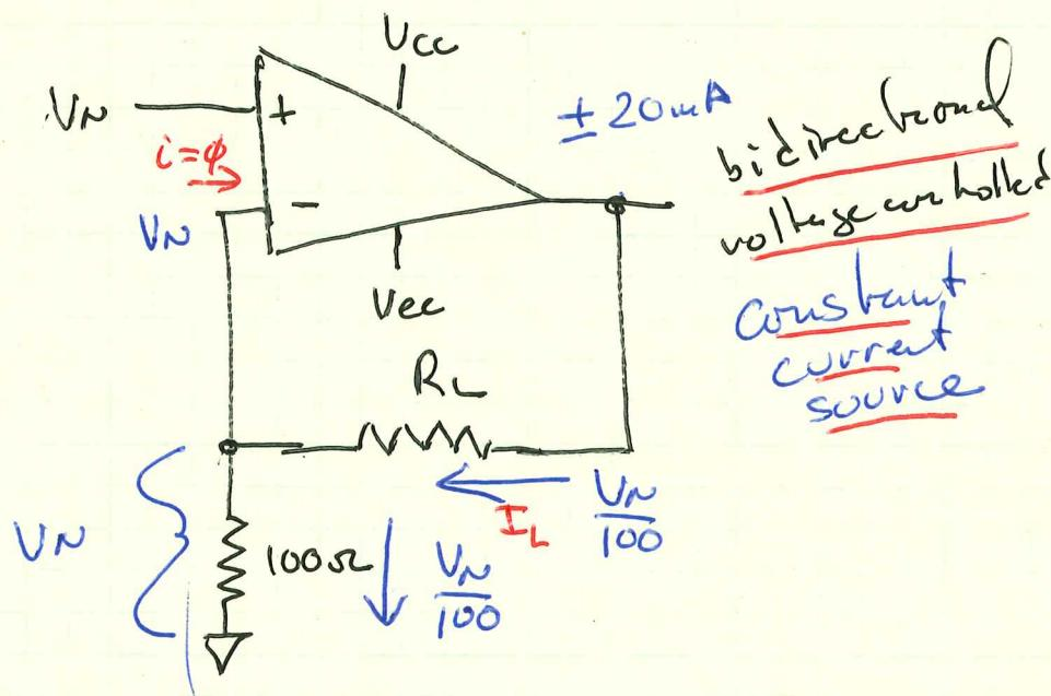
$$R_L \leq \frac{V_{cc} - V_N}{\text{max } I_L \text{ desired}}$$
