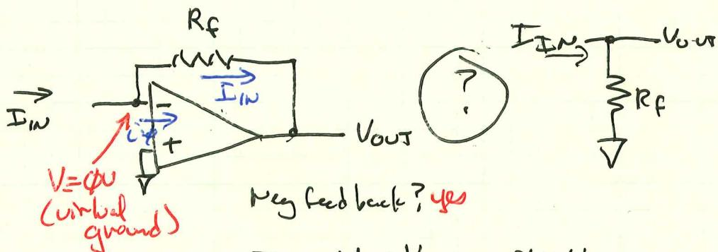
$$I_f = \frac{V - V_{out}}{R_f} = \frac{0V - V_{out}}{R_f}$$
