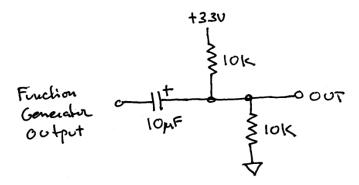
To analyze this circuit you need to remember that the impedance of a capacitor is inversely proportional to frequency. First consider the case where the input is DC (say zero volts for example). What would you expect the output to be? Build the circuit and test your intuition by applying 0V, -3.3V and +3.3V to the input. Does it matter what the DC voltage applied to the input is? (Hint: Yes it does but it is a physical limitation not a theoretical one. What is the physical limitation?)
