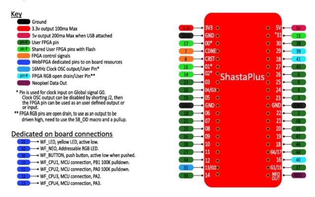
Suppose instead of the on-board LED, you wanted the white pushbutton to control an external LED connected between +3.3V and the WebFPGA board pin labeled "14" through a current limiting  $470\Omega$  resistor?
